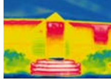
Building: Heat Loss
